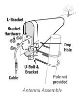
To install the outside antenna, assemble the u-bolt, bracket, nuts and washers as shown in the illustration. Keep the connections loose enough to allow the antenna to rotate until the optimum direction is found.
