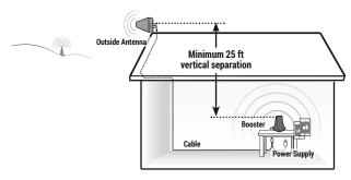
Before installation, ensure there will be adequate vertical separation between the planned locations of the outside antenna and booster (at least 25 ft.). Prior to securing the location of any booster parts, a "soft install" is recommended as adjustments may be needed to optimize performance.
