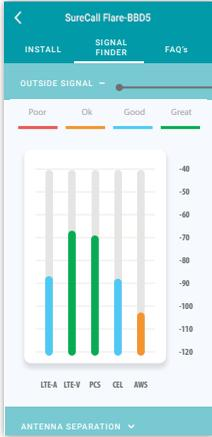
*When testing for the best placement and angle for your outside antenna, see "OUTSIDE SIGNAL" tab on the app.*
