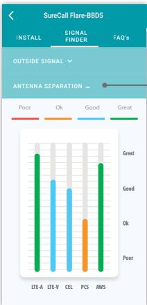
*Then get real-time feedback on your booster placement. See "ANTENNA SEPARATION" tab on the app to verify there's enough separation between the components.*
