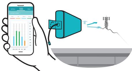
Performance is **LARGELY BASED ON** your outside signal **STRENGTH**. If signal is weak where the outside antenna is installed, indoor coverage will be limited.
